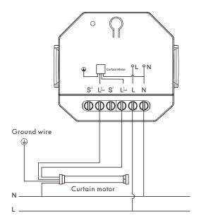
**Note:** The two push switches control the forward and reverse steering respectively, and the specific forward and reverse direction needs to be decided according to the actual curtain motor wiring.
